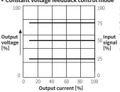
It outputs a constant voltage proportional to the control input so that the output voltage does not fluctuate against fluctuations in power voltage and load resistance fluctuations of loads (iron, chromium, signal nichrome, etc.) with a small electrical [%] resistance temperature coefficient.
