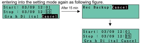
As data saving capacity of this recorder is 18138 ea, saving period is mentioned as next page according to recording mode.
