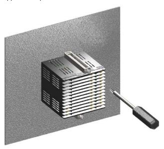
2nd Tighten fixing brackets on upper/lower parts to fix on the panel with screwdriver (+).
