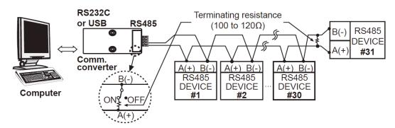
It is recommended to use SCM-US48I (USB to RS485 converter), SCM-38I (RS232C to RS485 converter), SCM-US (USB to Serial converter) of Autonics.
