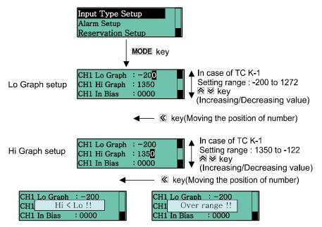
When High / Low graph setup with wrong value and pressing **MODE** key for save, error message is indicated as above.(Refer to Over Range, Hi < Lo of 8.2.4 Display information function (1) Error) Then if pressing **MODE** key again, it returns to previous value.
