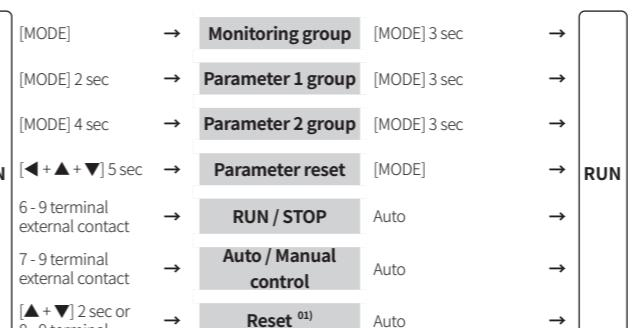
01) In the event of system anomalies and alarms, RESET input restarts the power controller. (parameters are not reset.)
